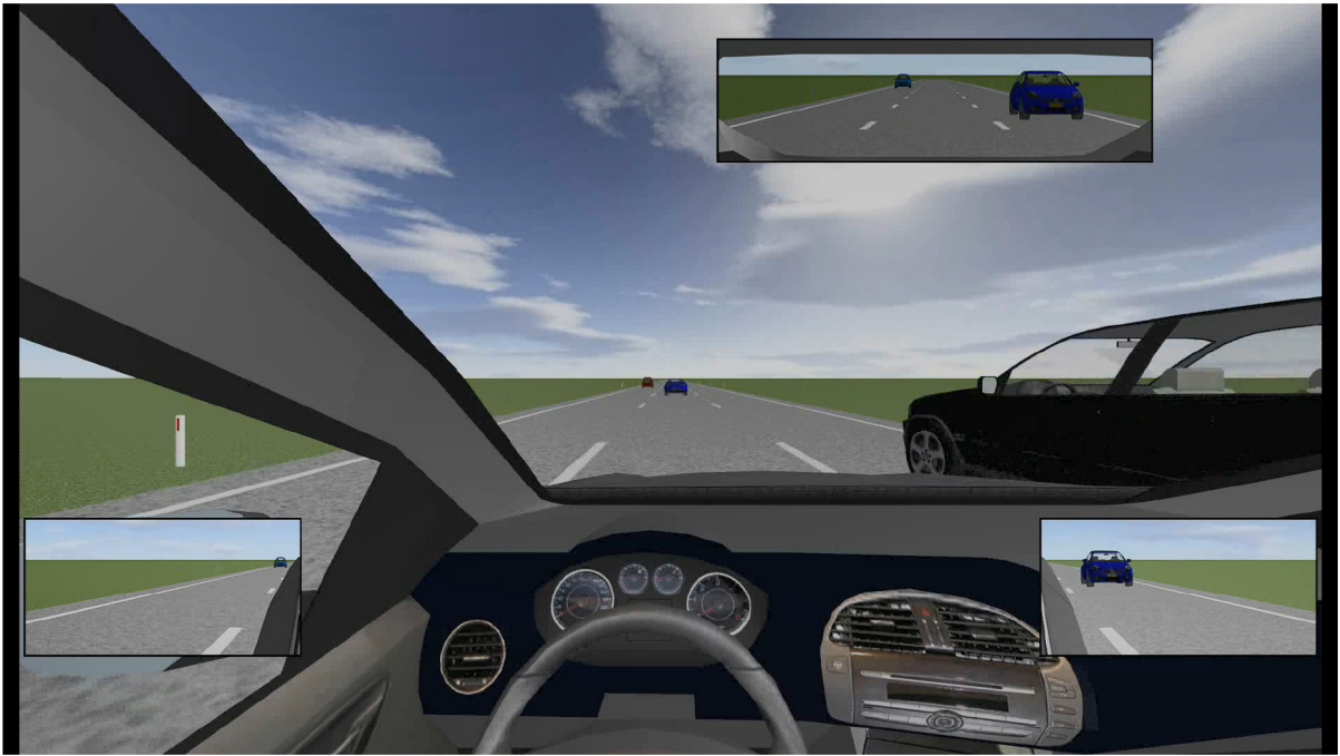
Fig. 1. The driving environment. In this hazard video, a car blocks the right lane. There is a stationary car in the ego-lane. Hence, the correct decision is to evade to the left. In total, there are five surrounding cars.
