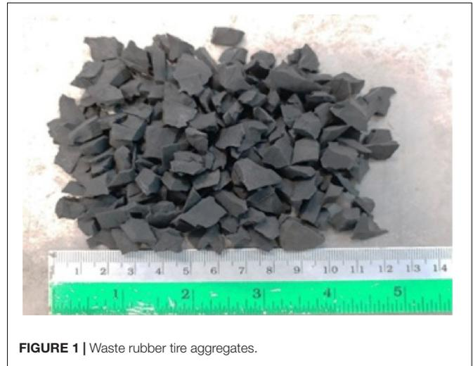
FIGURE 1 | Waste rubber tire aggregates.
