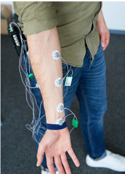
Figure 29. Placement of electrode to measure local muscle activity.
