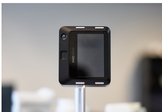
Figure 3. Photos of locating the center of gravity by balancing the separate components.
