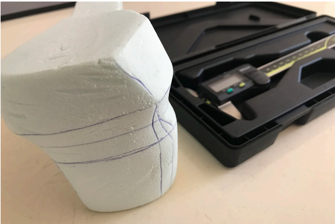
Figure 23. A digital calliper was used to measure the grip section for section. This formed a base for building a 3D loft in SolidWorks.
