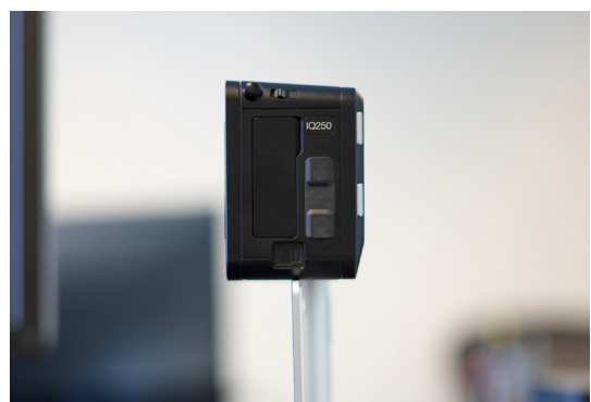
Figure 3. Photos of locating the center of gravity by balancing the separate components.
