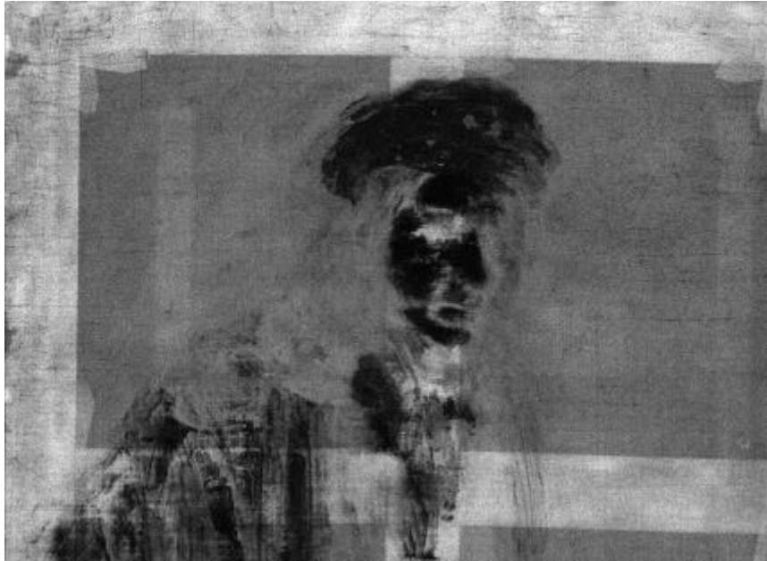
Figure 5: Compton scattering intensity map between 16.1 and 16.7 keV of 'Man with red baret'. It can be seen that the stretcher and the supporting beams give rise to a higher background radiation level. Even the easel which was used during the scanning of the painting can be observed. Secondly it can be seen that some sections are shielded due to lead-white presence in the paint layer.
