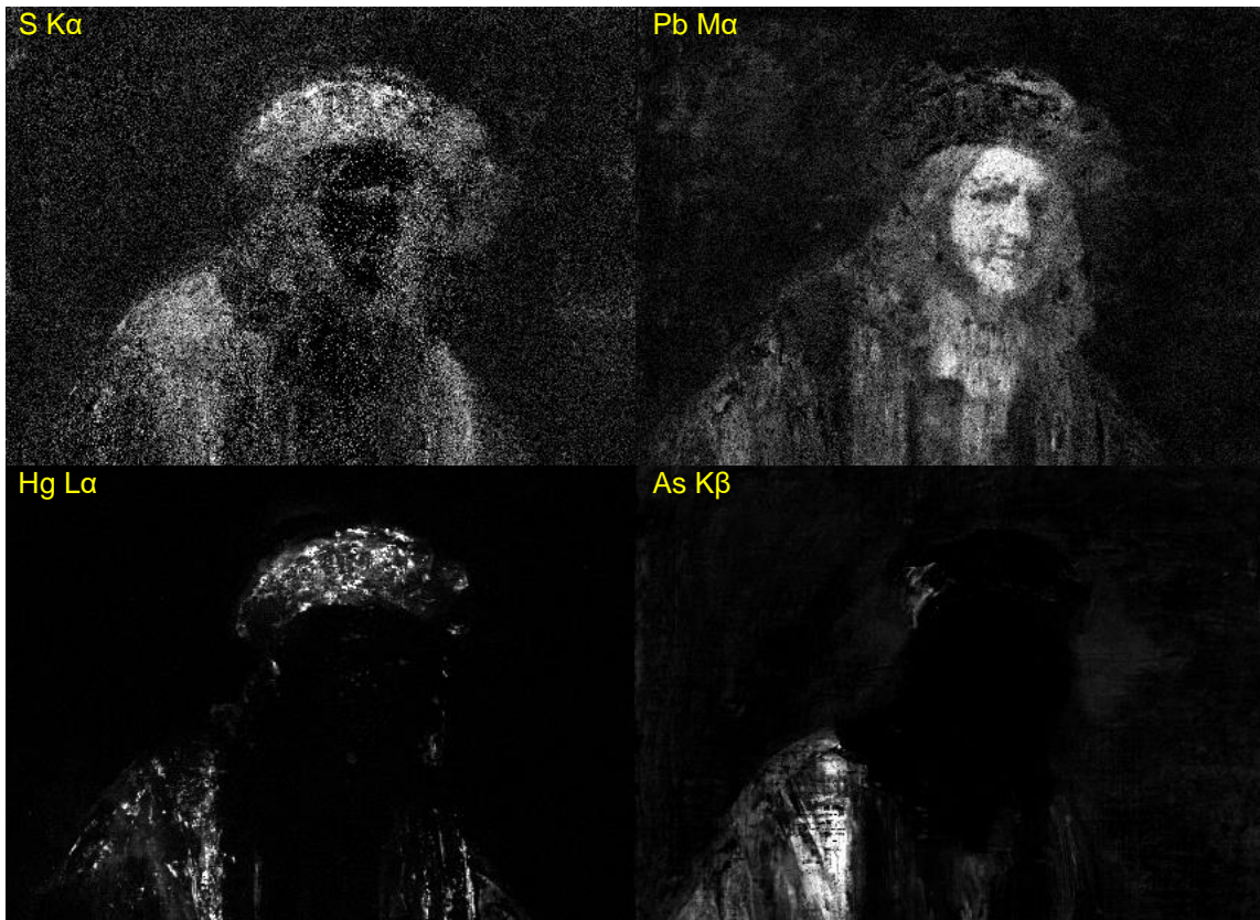
Figure 15: Comparison of the fitted S\ K\alpha and the Pb\ M\alpha peaks of the top part of the paintings. It can be seen that the S heavy parts are corresponding to the reddish parts of the painting itself which would correspond to the pigments vermillion ( HgS ) and Realgar ( As_4S_4 ), while the Pb rich parts are predominantly caused by lead-white at the surface.
