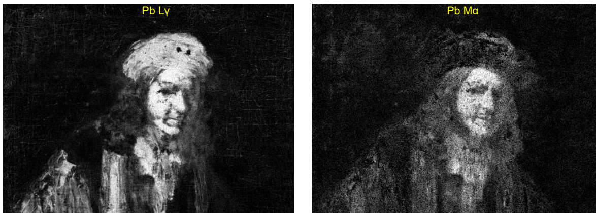
Figure 6: Comparison of the high energetic Pb Ly and low energetic Pb Ma elemental map. In the Pb Ly map the hat clearly shows the presence of lead, while in the Pb Ma no lead is detected. This suggests that the lead is to be found in deeper layers.
