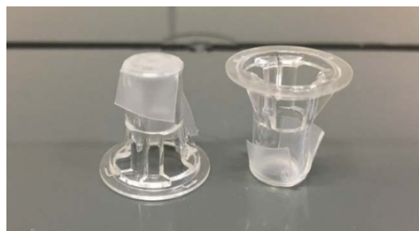
Figure 5 Transwell inserts covered with parafilm to prevent UPy-PEG leakage during neutralization.
