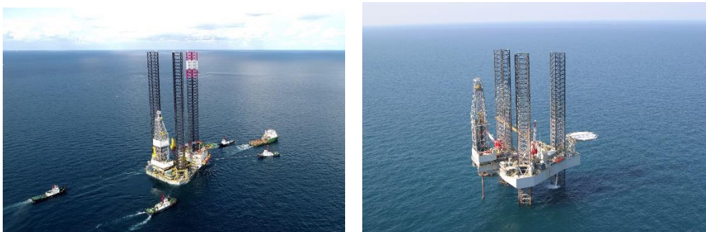
Figure 5.7 - Jack-up being towed and jack-up in-place [38]
