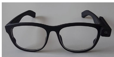
Fig. 3. The eye tracking glasses 'Pupil Invisible' of Pupil Labs.
