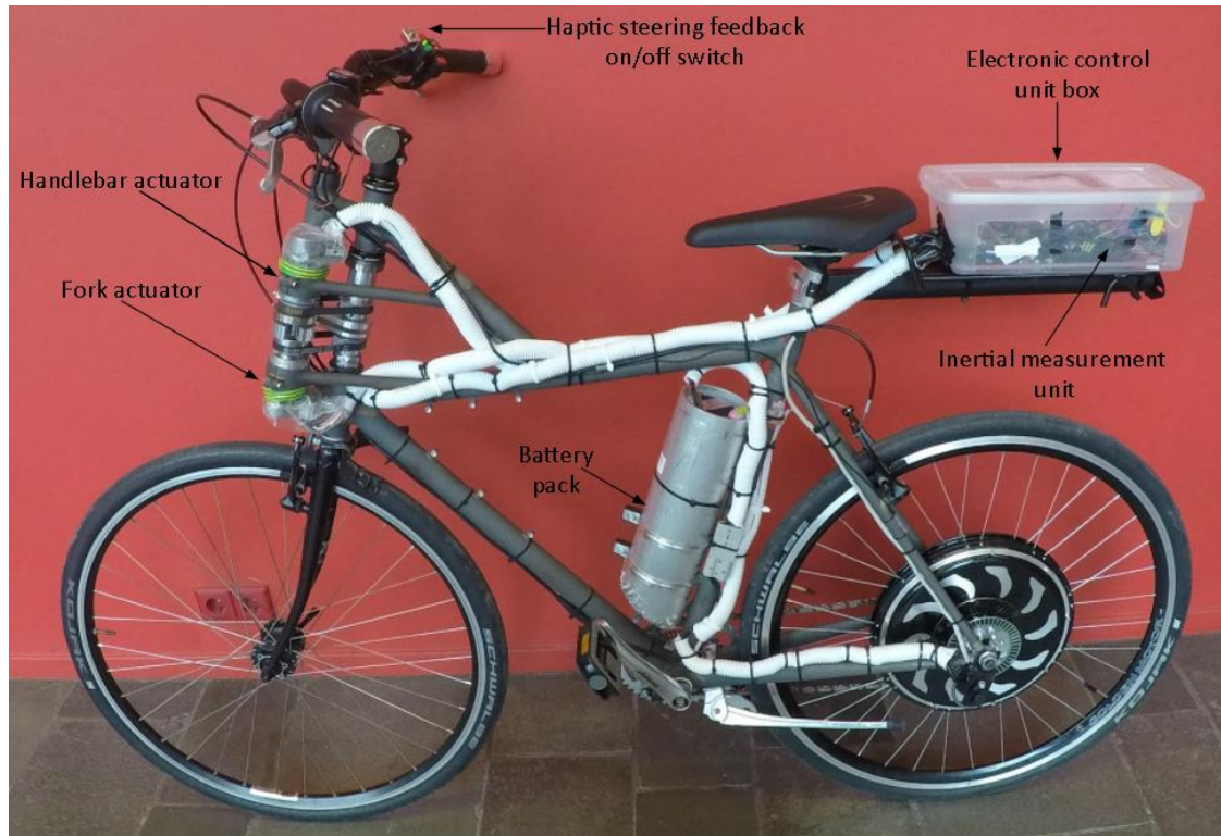
Figure 5. Prototype of the steer-by-wire bicycle with steering and handlebar actuators, sensors, digital controller and custom made battery pack.
