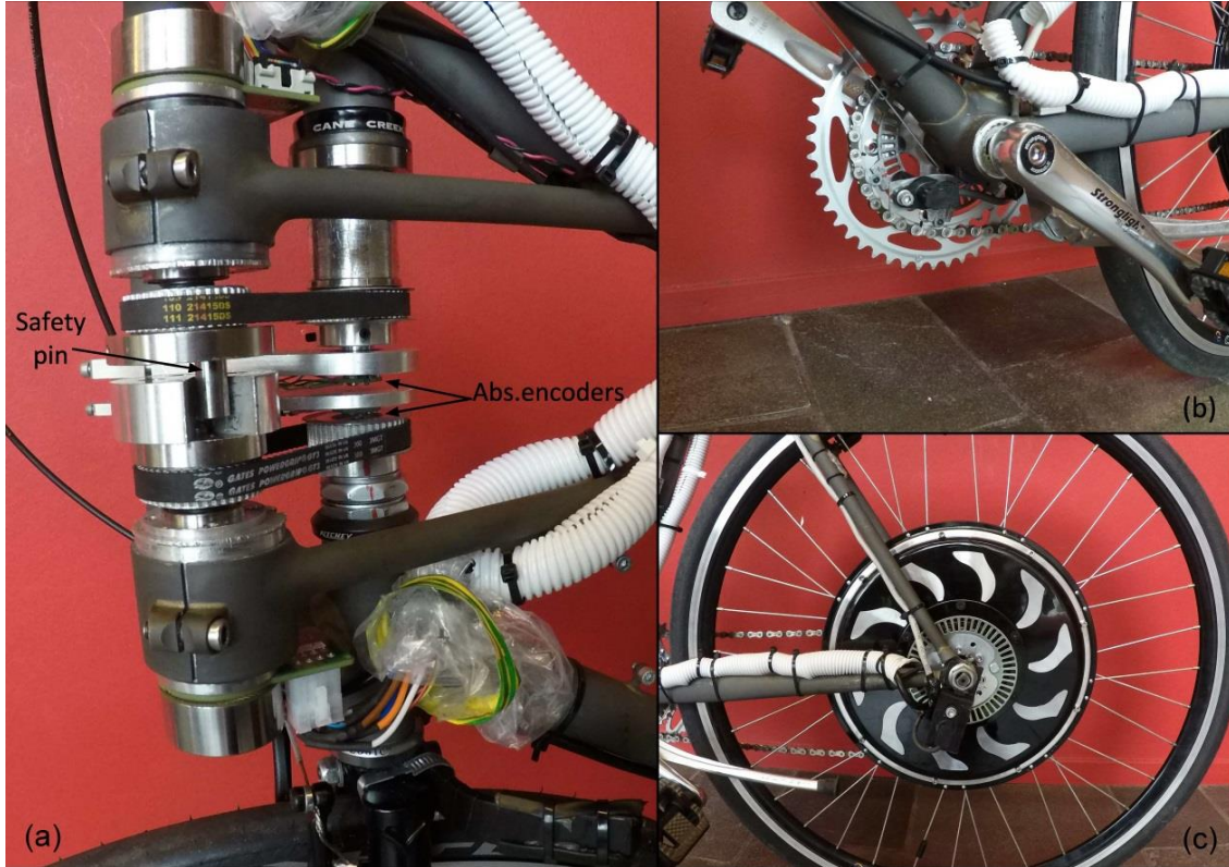
Figure 6. Steer-by-wire bicycle component layout, showing the physical placement of the actuators and sensors, with (a) headtube assembly with motor sensors and safety pin, (b) pedal speed sensor, and (c) rear wheel with forward speed sensor and hub motor.
