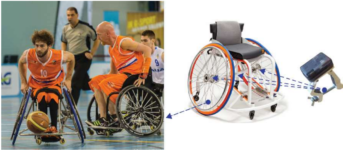
376 Figure 1. Measurement setup, with IMUs on wheels and frame and measurements during a match. (Photograph 377 by www.frankvanhollebeke.be ).
