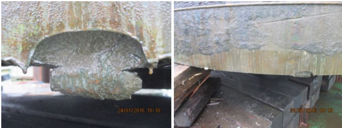
Figure 2.1: Uncut section of the Amrumbank met mast monopile.
