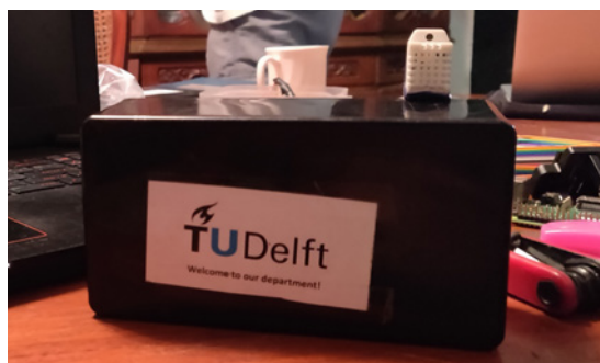
Figure 16: Final temperature and humidity monitoring device
