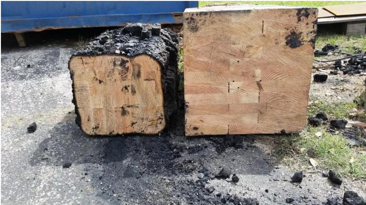
Figure 4: A slice of a glulam column after a standard fire test showing the reduced cross-section after a standard fire test of 90 minutes (Think Wood , 2023)
