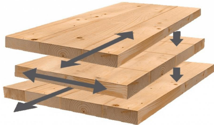
Figure 1: CLT panel lay-up (BY, 2018)
