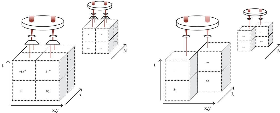
Figure 1. Visualization of multiplexing and diversity in the domains of time ( $t$ ), frequency ( $\lambda$ ), space ( $x, y$ ) and OGS sites ( $N$ ) for space-time block coding (*left*) and multi-beam, multi- $\lambda$  (*right*). Both schemes transmit – with the time-frequency-space-site bins shown – a total of 8 (complex) symbols and the transmission of symbols  $s_1$  and  $s_2$  are highlighted.
