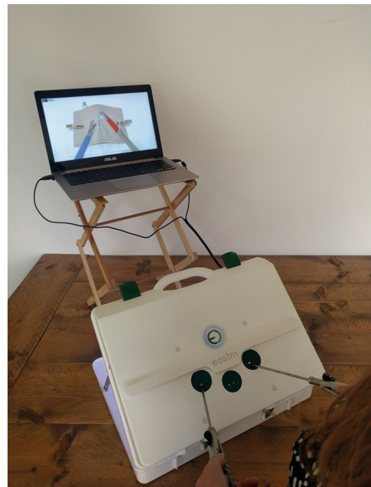
Fig. 1 The eoSim-augmented reality laparoscopic simulator interface
