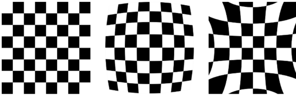
Figure 3-5: An image of a checkerboard captured with an ideal lens, a lens with positive distortion, and a lens with negative distortion, respectively. From [9].
