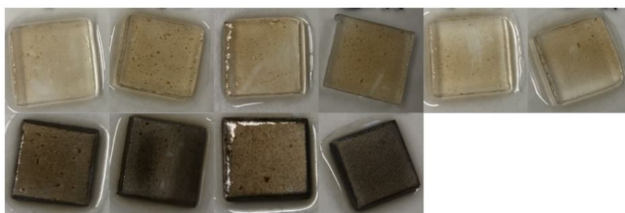
Figure 1.2: Biofilms formed by Cylindrotheca fusiformis on titanium and PMMA after 6 day immersion in a culture with a starting concentration of 8.0 \times 10^4 cells/mL [16]
