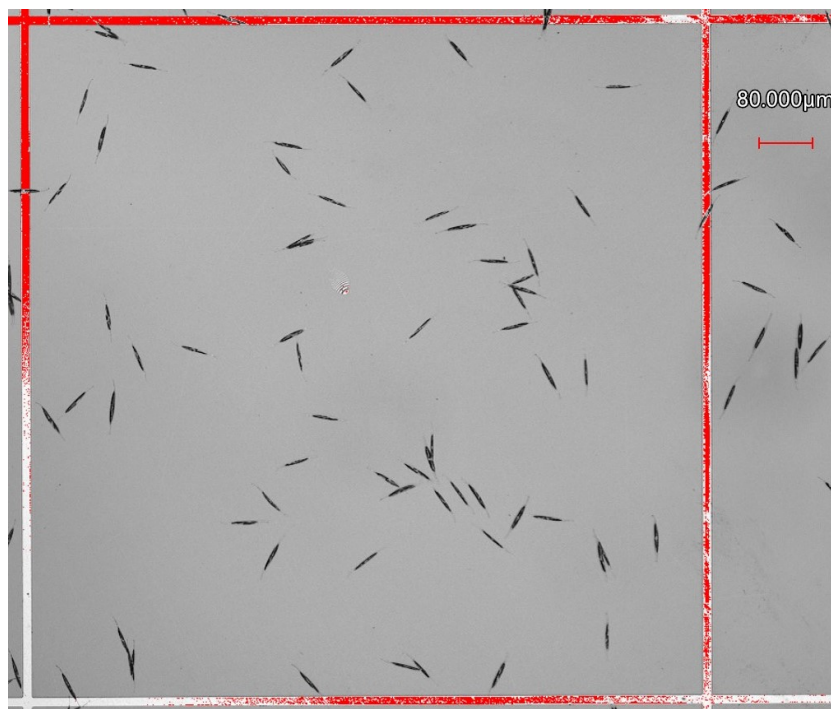
Figure 2.3: Example of a counting square under the Keyence Laser Scanning Confocal microscope in laser mode (mag: 10x)
