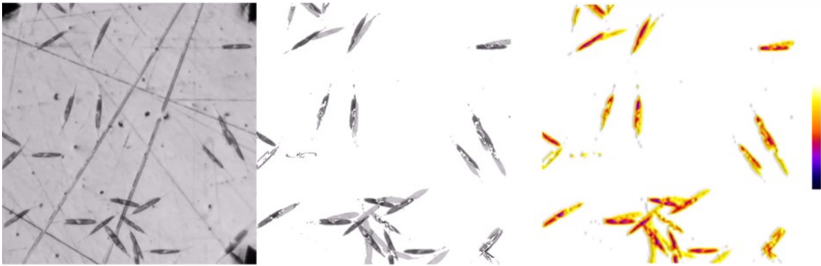
Figure 2.6: Frame from the image sequence produced by the general motility software; left shows the original picture in gray scale; the middle shows the changed pixels with respect to the previous image; the right shows the changed pixels with the color applied, a darker color implies a greater intensity change
