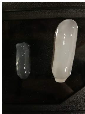
(a) Picture of how the artificial lymph nodes for batch one, two and three looked once removed from the mould
