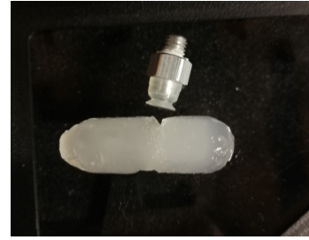
Figure A.3: Photo of the damage the 6mm suction cup inflicted on an Artificial node from batch 1
