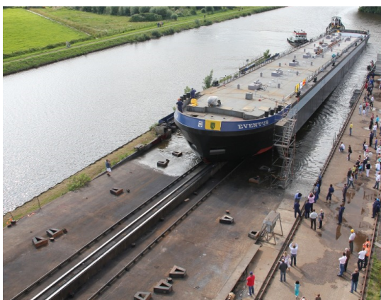
Figure 1.10: End launch of a ship. Image is from: (GS Yard, 2010).
