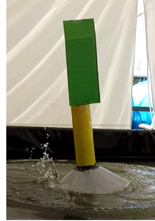
Figure 4.13: The GBF returns to its upright position and causes a splash at the back.
