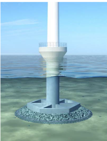
Figure 1.3: Flat based, open caisson GBF. (Energinet.dk, 2015)
