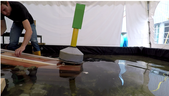
Figure 4.2: Overview image (camera 1) of the testing facility with the inclined slipway and the GBF scale model. The space on the right was used for the free decay tests.
