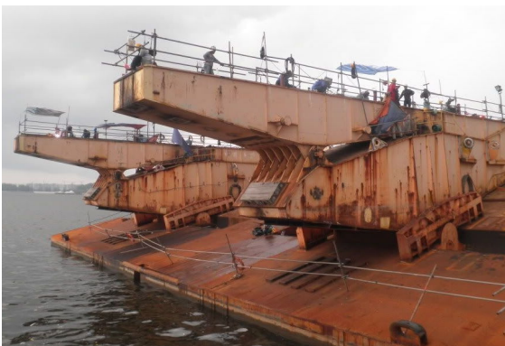
Figure 1.15: Rocker arm on a barge used to distribute tipping loads when launching jackets. Image is from: (ombugge, 2016).
