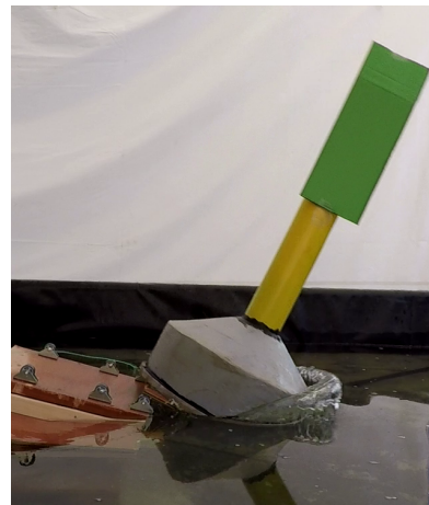
Figure 1: Image of a gravitational launch of a GBF during an experiment performed for this thesis.
