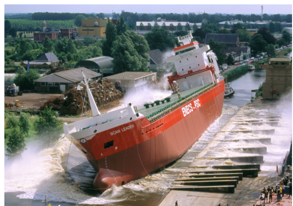
Figure 1.11: Side launch of a ship. Image is from: (Slater, 2016).
