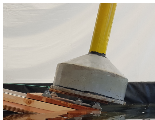
Figure 4.3: Image of the GBF on the slipway inclined at 14^\circ , with a +4 cm freeboard height and released from the low position.
