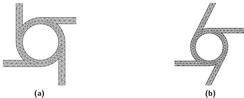
Figure 3-4: Meshes used for the simulation of Sample A.1(a) and A.2(b)
