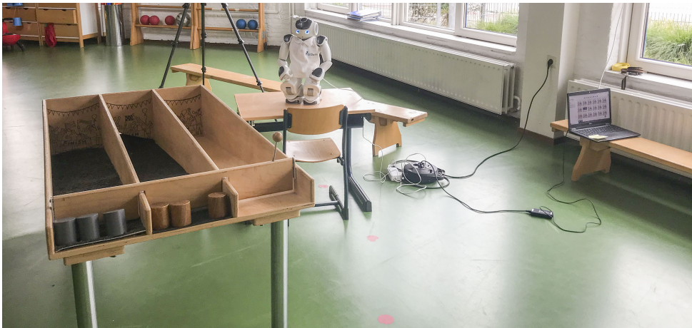
Figure 5.1: The 'rolling-rolling' exhibit in the present study set-up. This exhibit allows children to investigate the effect of roller weight and surface material on rolling speed by rolling two or more rollers down (starting simultaneously by using the lever) and observing rolling speed.
