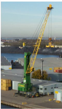
Figure 2.3: Mobile grab crane for unloading vessels. Source: Verbrugge (2020)
