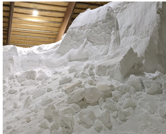
Figure 3.3: The formation of clumps due to the absorption of moisture
