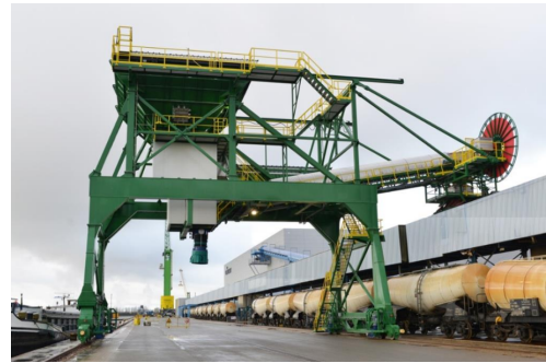
Figure 2.5: RM hopper for receiving bulk material discharged by grabs. Source: Verbrugge (2024)
