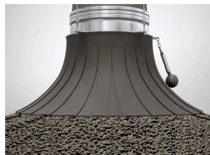
Figure 5.7: A dust skirt at the outlet of a loading chute. Source: Vortex (2022)
