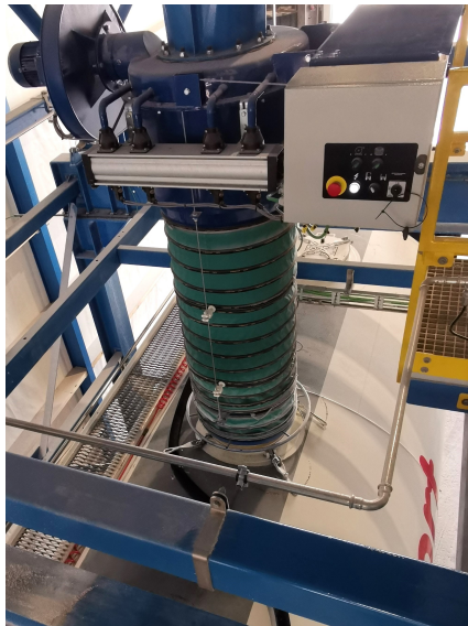
Figure 6.1: Telescopic chute attached to hatch of a truck
