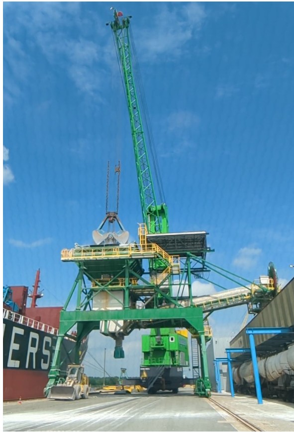
Figure 8.3: Transfer between the grab and RM hopper at Verbrugge
