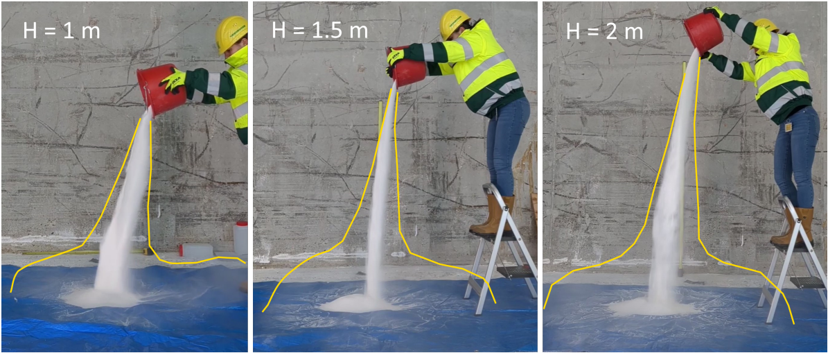
(d) Visible dust dispersion during drop test 3
