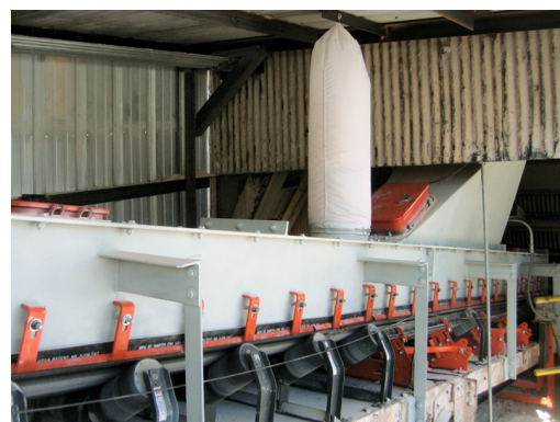
Figure 5.12: Dust bag. Source: Swinderman et al. (2009)
