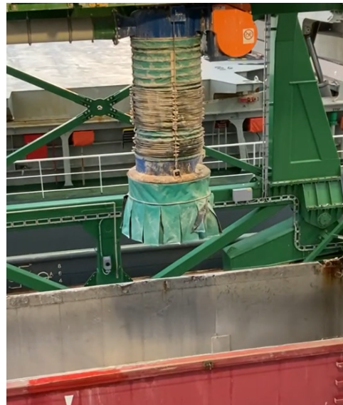
Figure 6.2: Telescopic chute with outlet dust skirt. Source: Verbrugge (2024)
