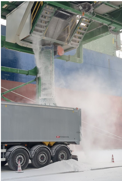
Figure 6.8: Observation of telescopic chute with dust skirt during loading of an open truck
