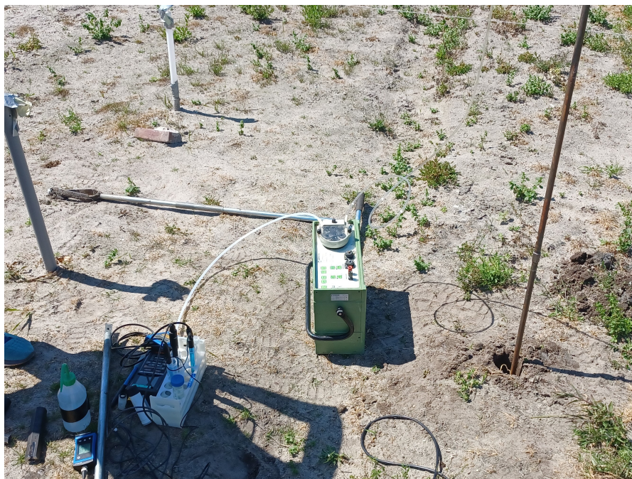
Figure 2.8: Overview of groundwater sampling with the GVP. The iron tube on the right is the GVP from which the water is taken with the peristaltic pump. On the left are the Greiner tubes with the EC, Ph and redox devices.
