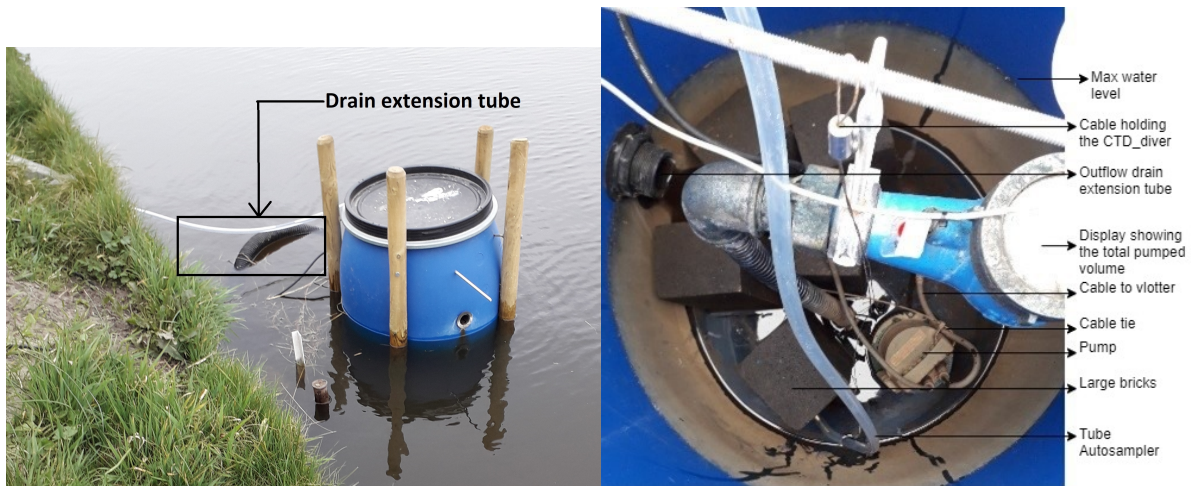
(a) View of B1 from the outside. The drain is connected to B1 with a drain extension tube that floats on the water level of the ditch. Therefore D1 has to overcome the water pressure of the ditch before it can flow into B1. In this way, the water level in the ditch is simulated to create a natural drain response.
