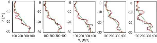
**Figure 6.** Inverted 1-D  $V_s$  profiles to check the accuracy and resolution of FWI to capture the lateral variability in the soil: the black lines denote the true  $V_s$  values at the locations of the SCPTs, the green lines are the initial  $V_s$  values (same at all locations), and the red lines are the inverted  $V_s$  values, using the pseudo-observed seismic data.
