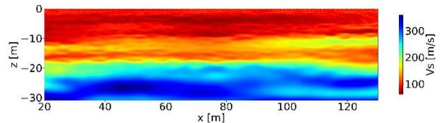
**Figure 4.** Inverted 2-D velocity model by FWI.
