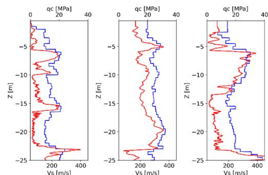
**Figure 1.** SCPTs from Groningen, the Netherlands (<https://www.dinoloket.nl/>). The blue lines denote the  $V_s$  values, and the red lines are the  $q_c$  values at the same location.
