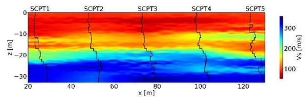
**Figure 2.** The “true”  $V_s$  model obtained by interpolating between 5 actual SCPTs. This model is used to derive the pseudo-observed seismic data. The horizontal separation between the SCPTs is 25 meters.
