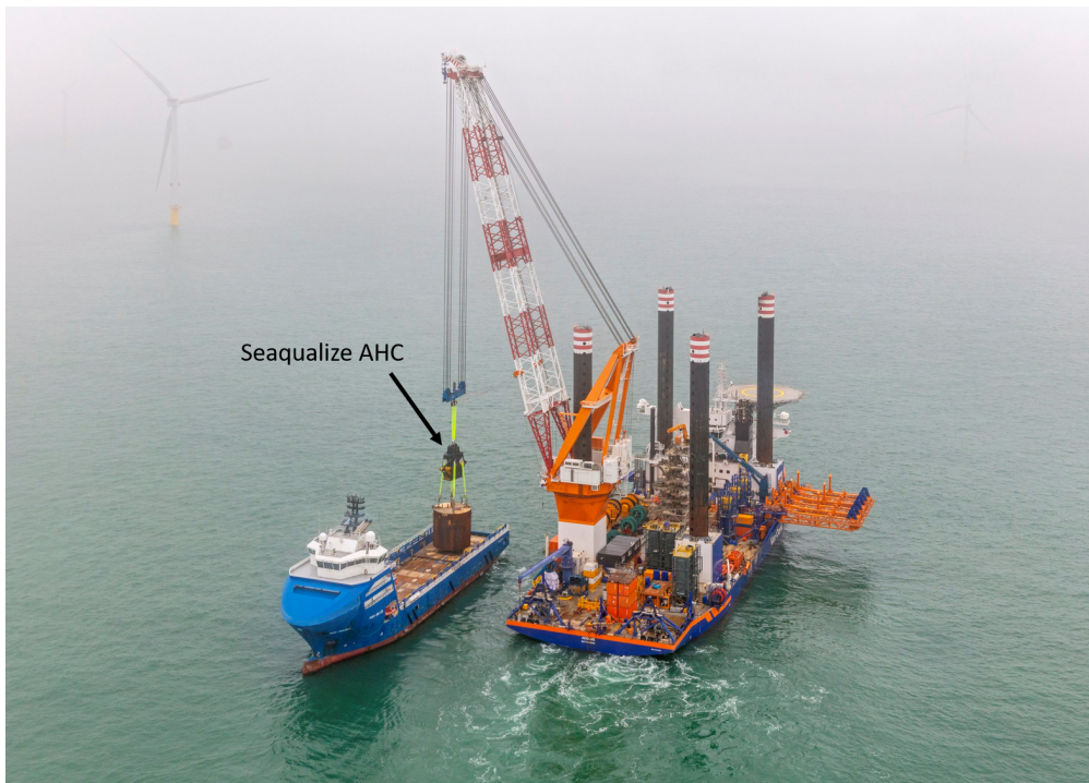
Figure 2.22: Sea trials (lifting tests) of the AHC tool of Seaqualize (Seaqualize, 2022)
