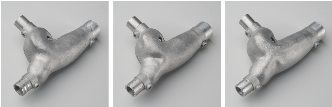
(a) Optimised manifold printed at an angle of 45^\circ
