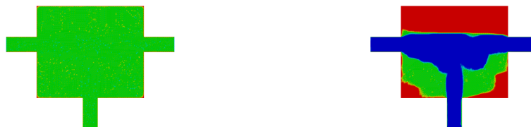
(a) Design field if there is a no or a very low greyness constraint (b) Design field if there is a small valued greyness constraint
