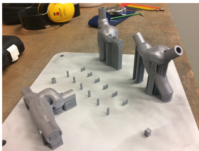
Figure 6.1: Manifolds on the build plate with external support material
