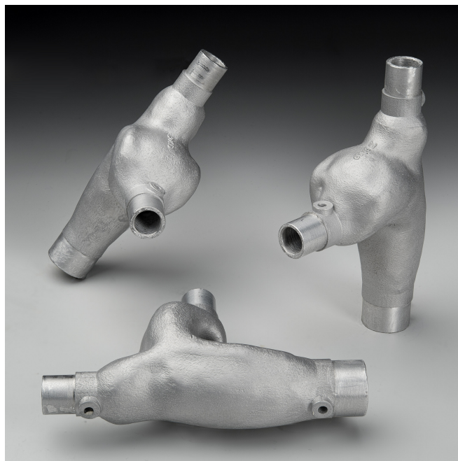
Figure 6.4: All three manifolds displayed in their printed orientation
