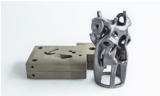
Fig. 3 TO steel node cast on 3D-printed sand mould by Arup and 3Dealise. Image credits: Arup/ Davidfotografie
