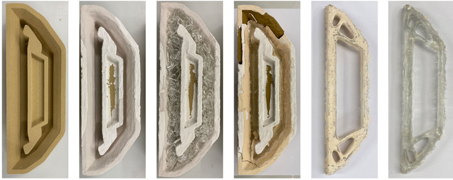
Fig. 10 Geometry 3, sample CCSX2F4a. From sand mould to glass piece. From left to right: 1. 3DPSM geometry, 2. Crystalcast® protective layer (3x, Brush), drying time: 3 days (ambient temperature) and coating application (Zirkofluid® 6672, 2X flow), drying time: 1.5 h between each layer, 3. Glass cullet placement, 4. Mould after firing at 870 °C normal schedule, 5. Cast glass part after demoulding, sand can be easily scooped out with the use of a soft brush but coating requires more tools, 6. Final glass elements after cleaning with the help of a rotary tool (Dremel®) and a sponge using water and isopropanol (top surface)
