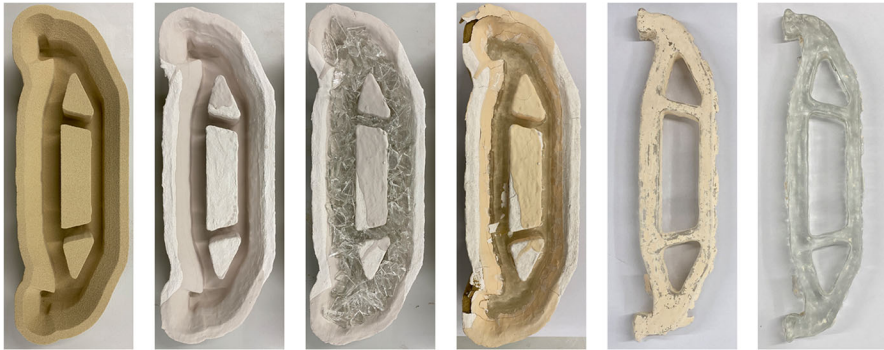
Fig. 11 Geometry 4, sample CCSX2F4b. From sand mould to glass piece. Same steps as in Fig. 10
