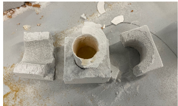
Fig. 9 Thin-shell distinct mould formed by the protective layer of Crystalcast® on quartz sand mould after firing at 970 °C normal
