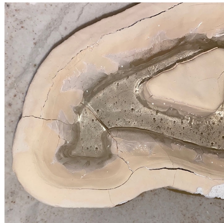
Fig. 12 Geometries 3 (sample CCSX2F4a, front) and 4 (sample CCSX2F4b, back) after cleaning with a soft metal brush attached to a Dremel®, contact side
