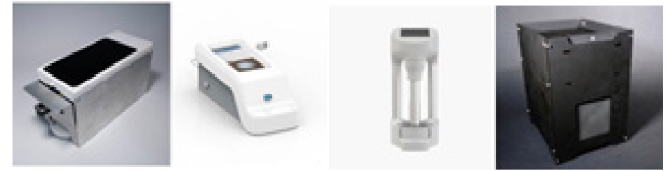
Figure 3. Mobile phone and Raspberry Pi based Schistoscopes.
