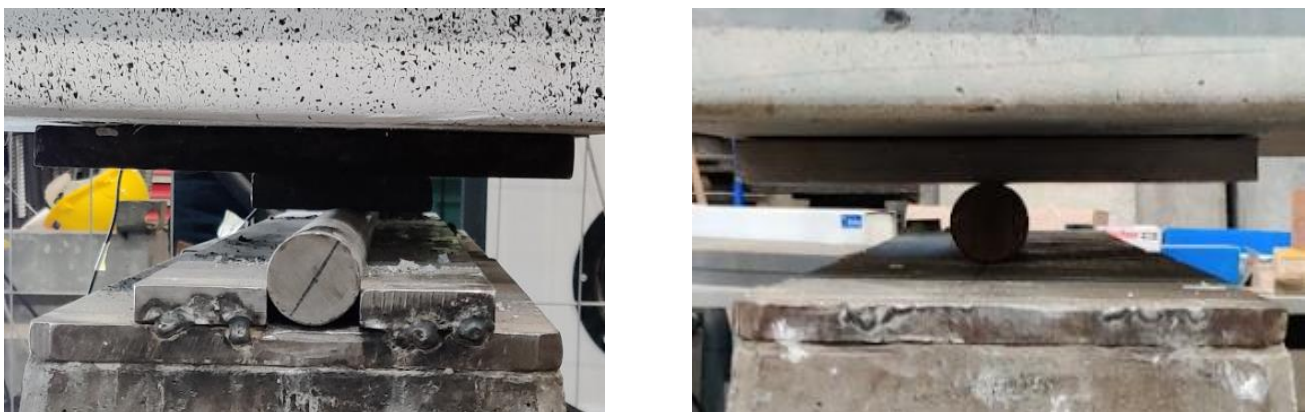
Figure 3-24: Picture examples of the blocked roller, and roller support with a metal plate between girder and supports, visible is the thin layer of mortar between the steel plate and girder.
