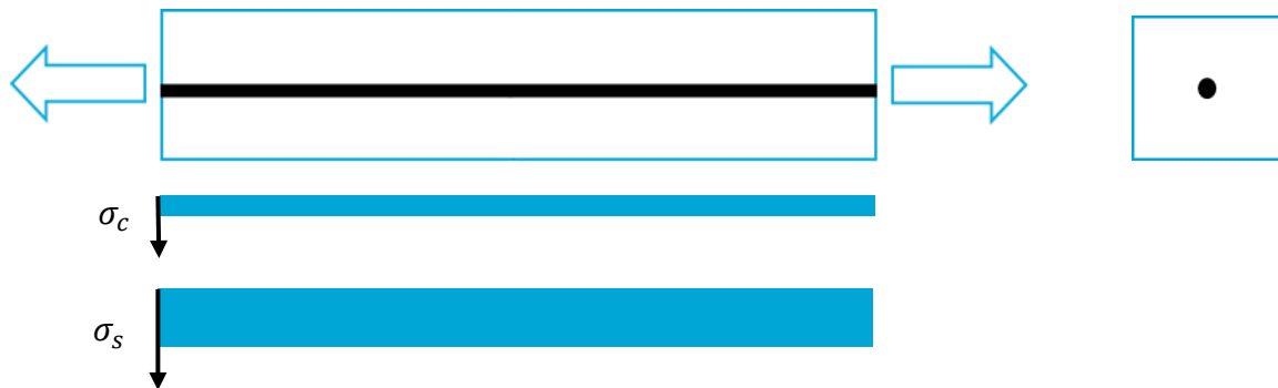
Figure 2-4: Tensile chord model where no cracking is present, concrete strain is equal to steel strain
