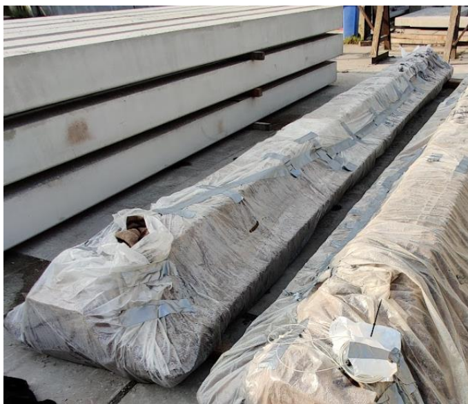
Figure 3-2: Open storage of 2 girders at Haitsma Beton's yard, wrapped in burlap cloth and plastic
