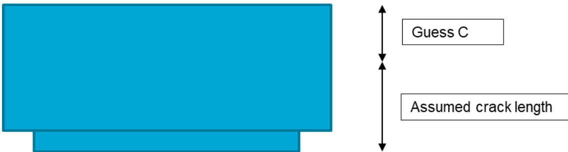
Figure 4-27: Cross section with the guessed location of the neutral axis: distance C. Prestressing strands are not shown for simplicity, for strand locations, see Figure 3-6
