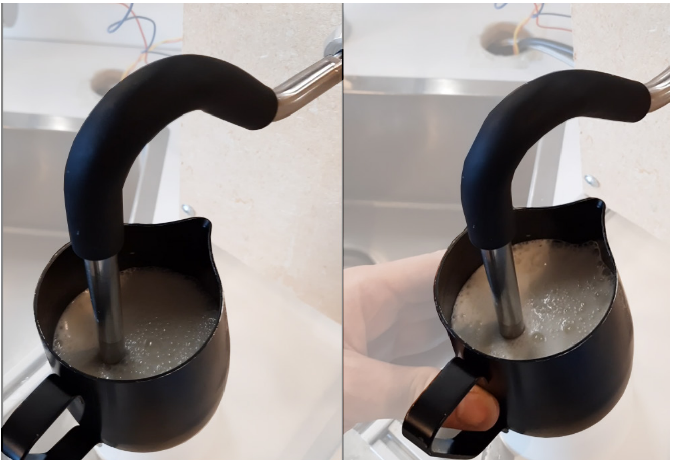
Figure 100 : Volume increase in the milk by using the venturi injector
