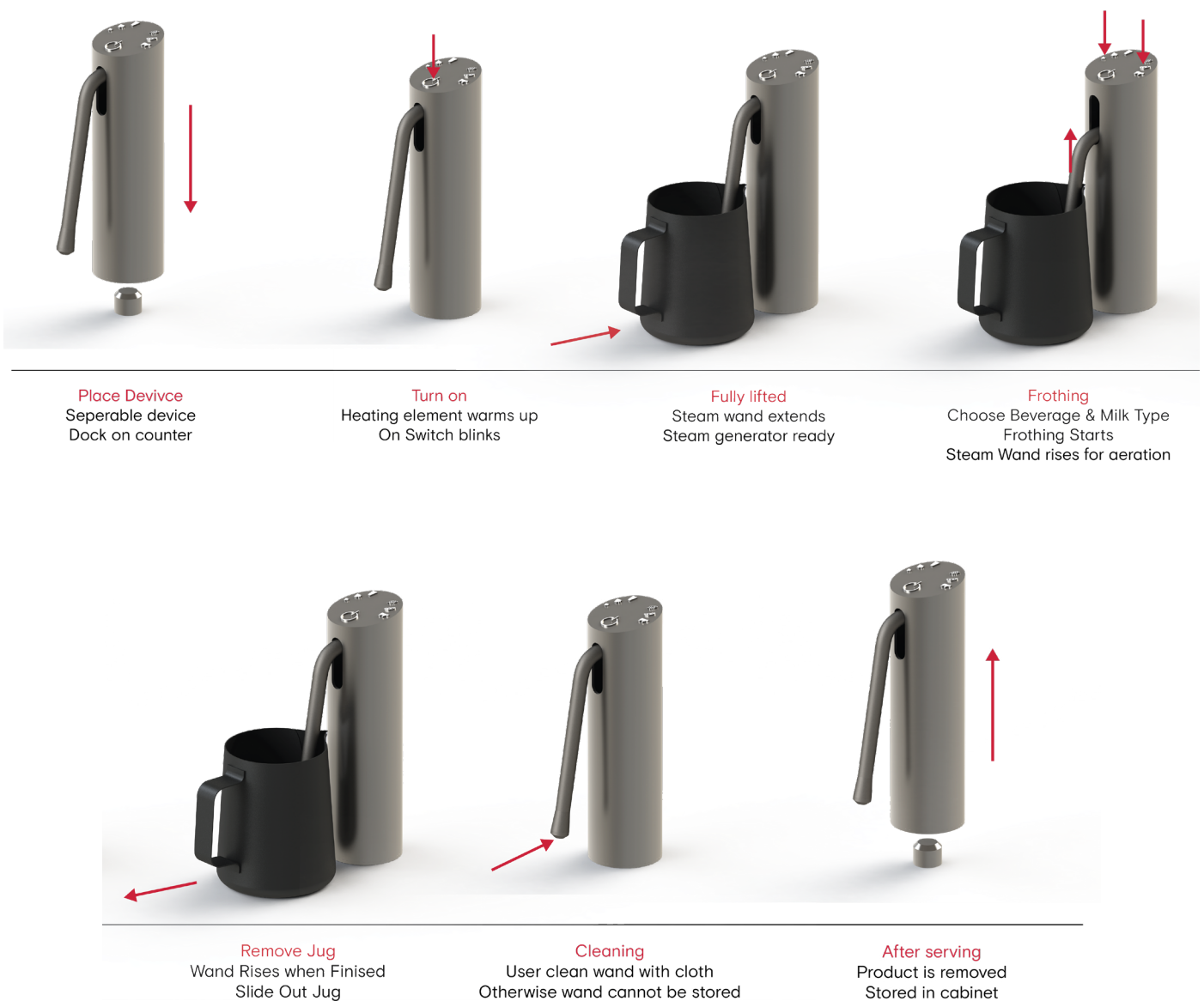
Figure 44 : Concept 3 frothing process
