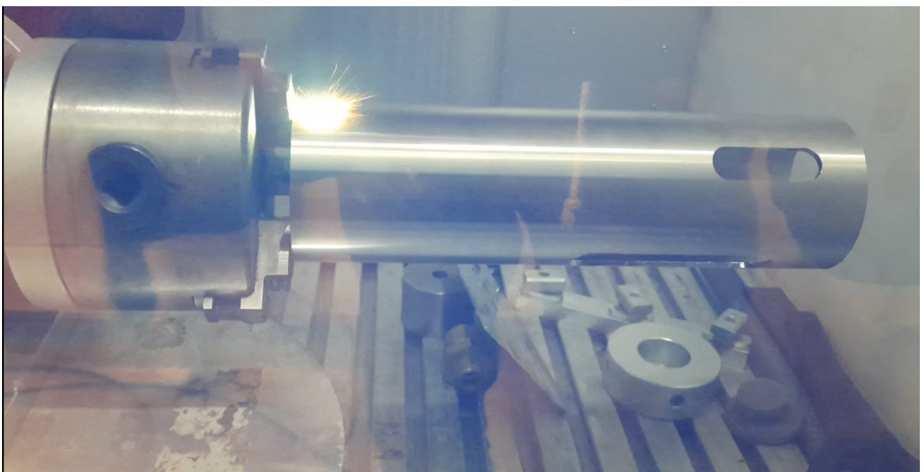
Figure 105 : Engraving process of the stainless steel tube
