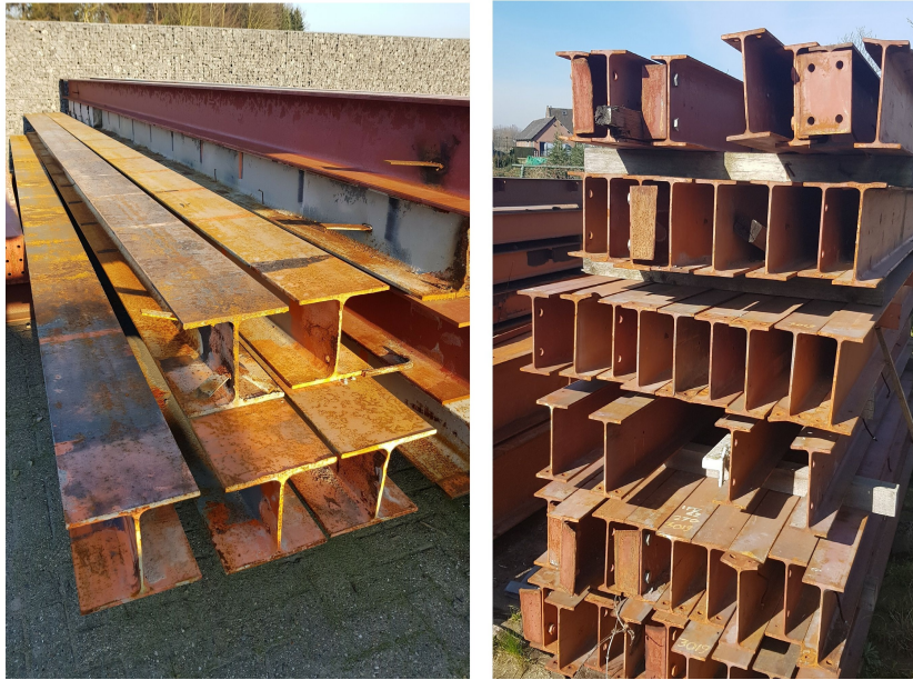
Figure 2.2: Pictures from van Liempd (2024) their available stock of HEA300 and IPE220 beams. As can be seen in the image, the elements are stored outside which will result in the need for a thorough visual check as per NTA8713. For the sake of this research, the quality of the beams is assumed to be fit for reuse, but it is important to note this is not a guarantee with this type of source.
