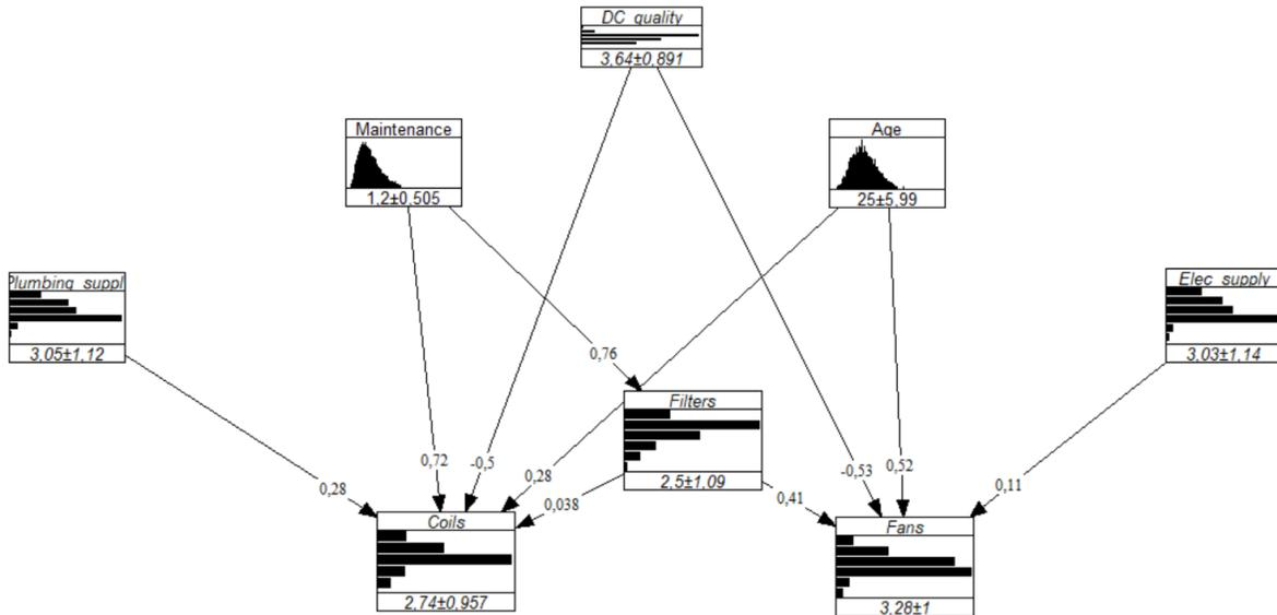
Figure 6.2: Quantified NPBN for the estimate of air handling units' condition.
