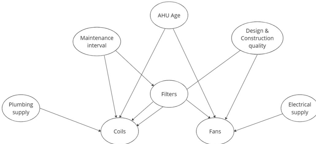
Figure 4.3: Graph structure for the air handling unit.
