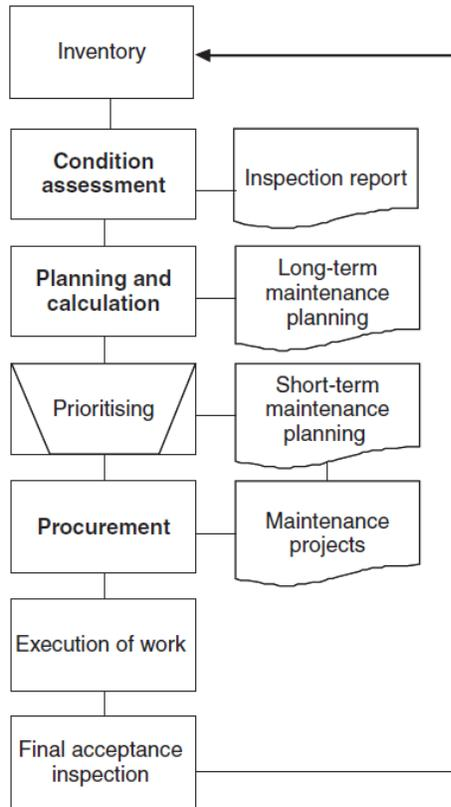
Figure 1.2: Condition-based maintenance process (Straub, 2012).
