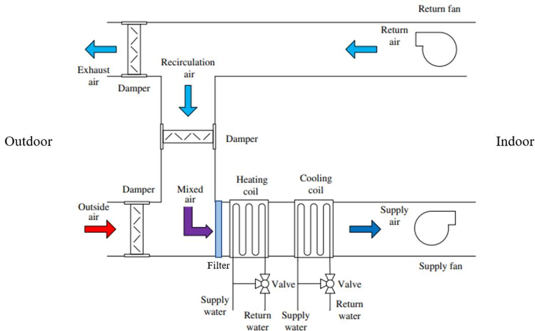
Figure 4.1: Air handling unit with air recirculation (adapted from [Kusiak & Li, 2010](#)).
