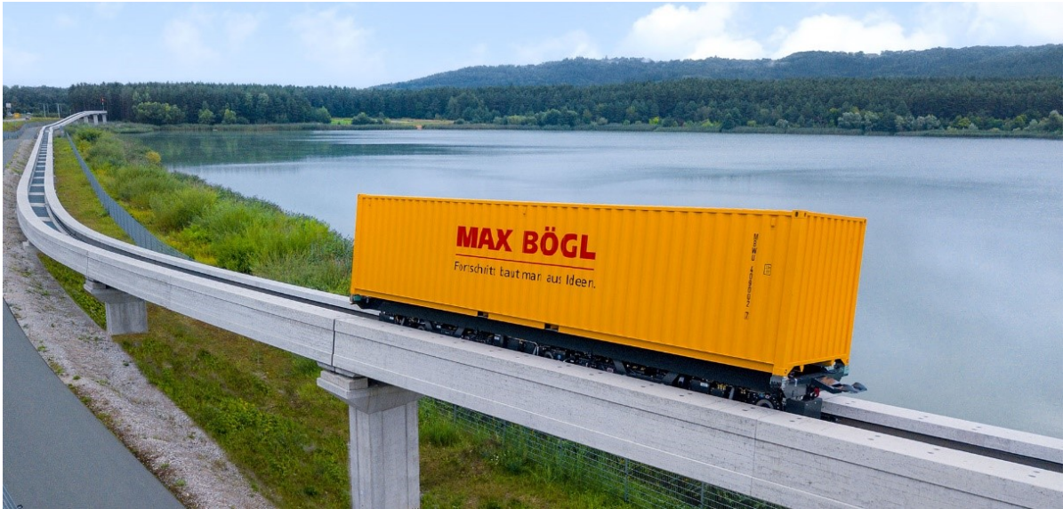
Figure 1.2: TSB Cargo, the maglev transport system from Max Bögl at the 860-meter test track in Sengenthal (Germany) . Source: Bögl, 2021.
