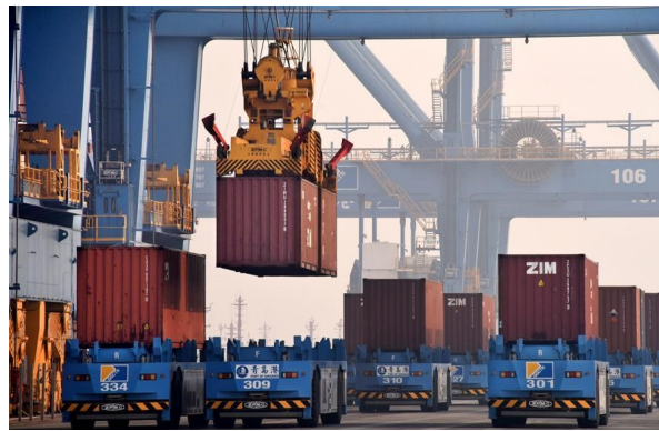
Figure 2.3: Cargo containers are transferred from QCs to AGVs at a fully automated container terminal of the Port of Qingdao in east China's Shandong Province. ( Xinhua, 2018).
