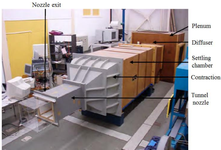
Fig. 3.1. Photo of W-tunnel in the Aerodynamics Laboratories at TU Delft.
