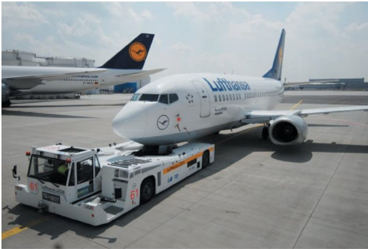
Figure 2.2: TaxiBot in operation at Frankfurt Airport [157].
