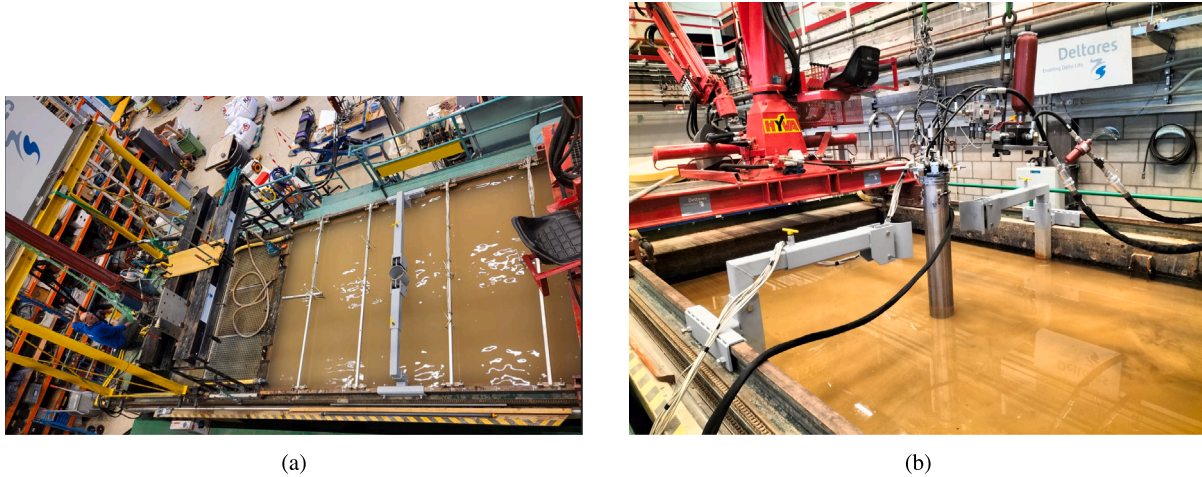
Fig. 4. The GeoModel container of dimensions 4 \times 2.5 \times 1.2 m at the GeoLab of the Deltares facilities in The Netherlands.
