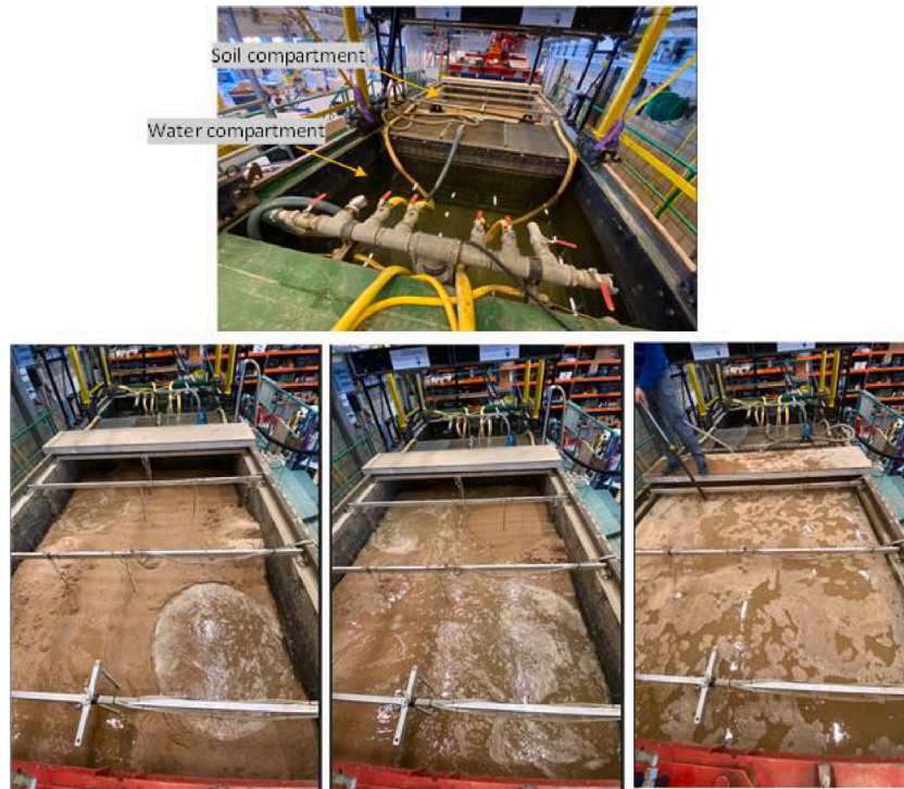
Fig. 7. Water saturation of the sand bed in the GeoModel container.
