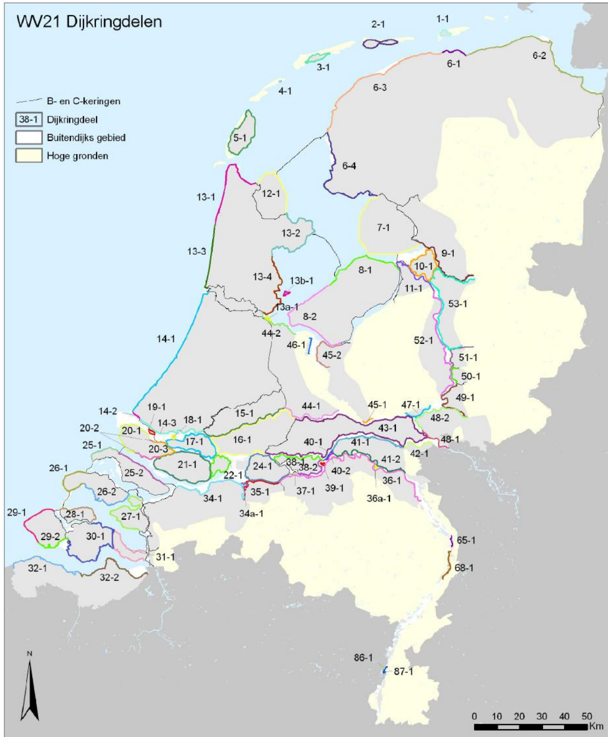
Figure A.3: In this figure, all dike-rings and dike-ring sections are shown. 14-1 stands for dike ring 14, section 1. From this figure one can see the large amount of flood defences through the Netherlands. From: de Bruijn and van der Doef [2011].
