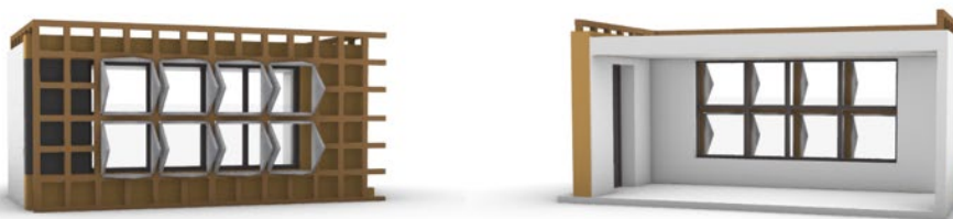
Figure 45: Kinetic shading system in façade when opened, made by author.
