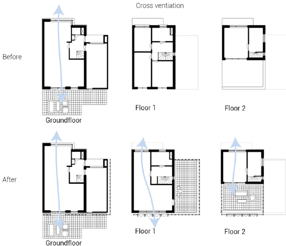
Figure 49: Opening the windows and doors to support cross ventilation through the building, made by author.
