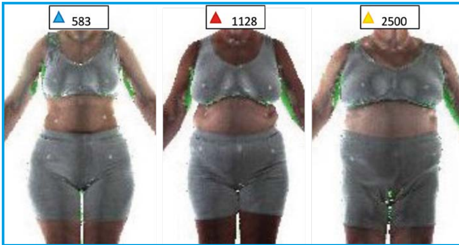
Figure 3.1 Scanned data from three figures of similar height and weight but with different circumferences, hence body shape, are shown with measurements and means of the subset ( n=100 ). Circumferences are in millimetres and weight in kilograms.
