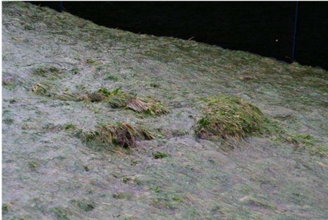
Figure A.4: Boonweg, section 4. Slope failure during a simulation with a load of 75 l/s/m overtopping waves. Development of a protruding bulge filled with water. Bulge withstood overtopping waves for 5 minutes before bursting.
