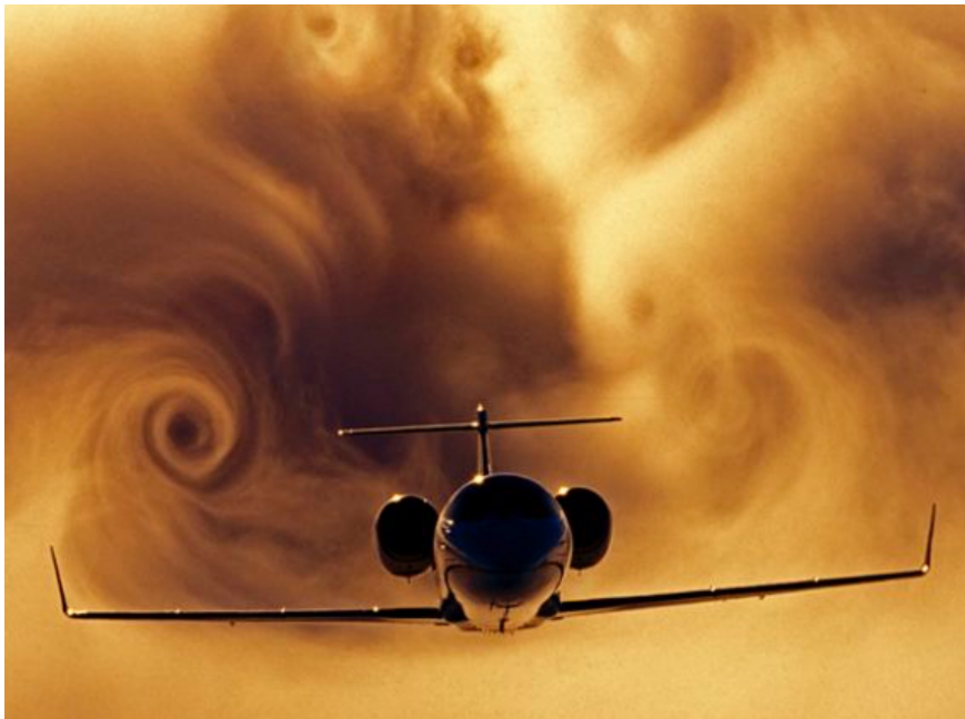
Figure 1.1: Wake vortices visible in the clouds. Photo credits: Paul Bowen, Cessna Aircraft Company.
