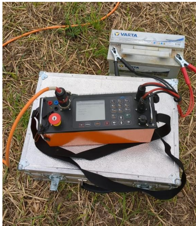
Figure 37: ERT measuring device and battery power source
