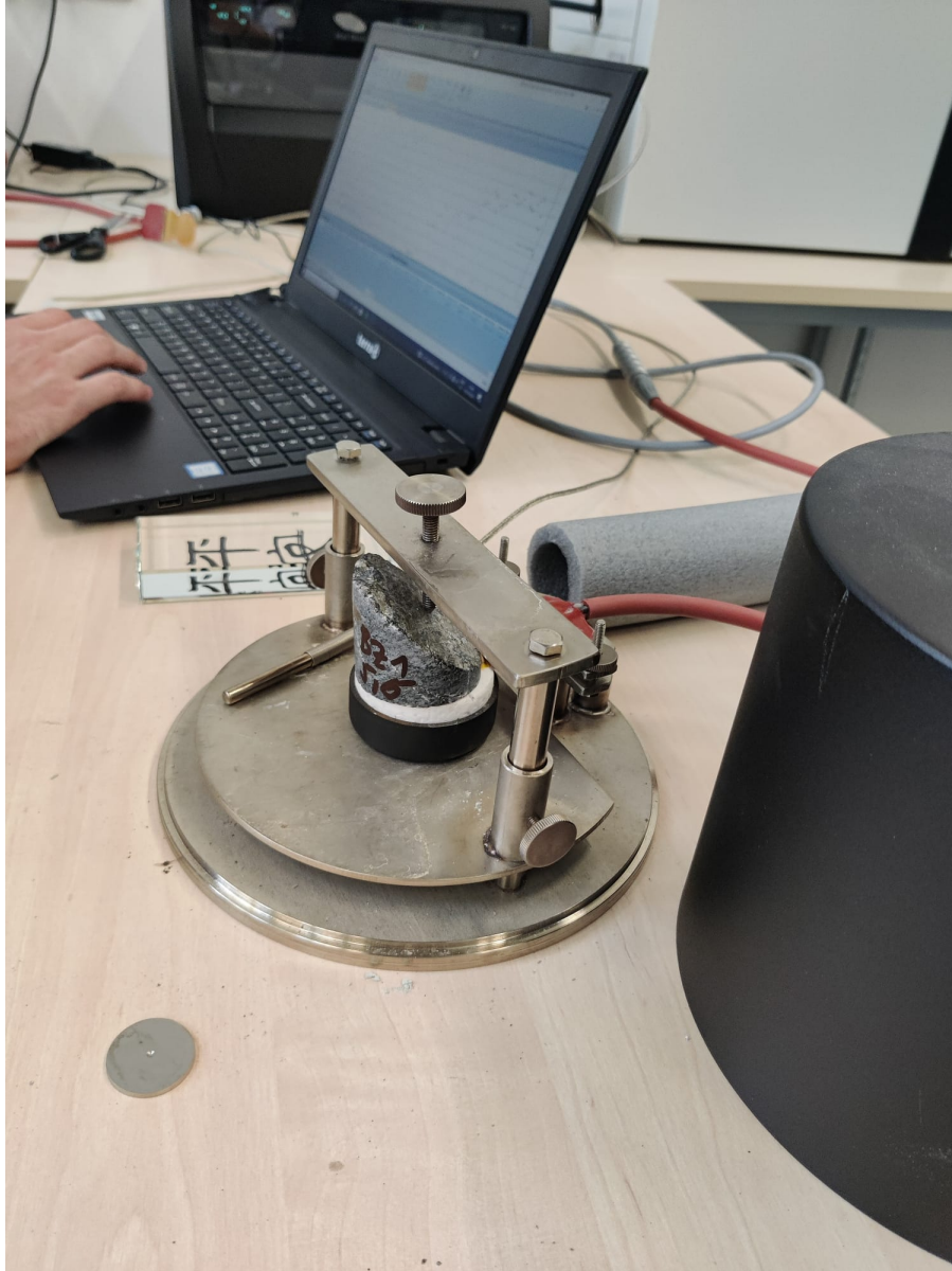
Figure 66: The hot disk device conducting a single sided measurement with sensor between rock sample and insulating styrofoam.
