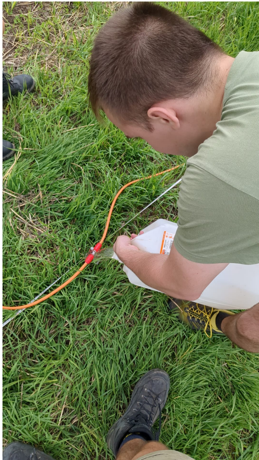
Figure 39: Wetting soil around electrode
