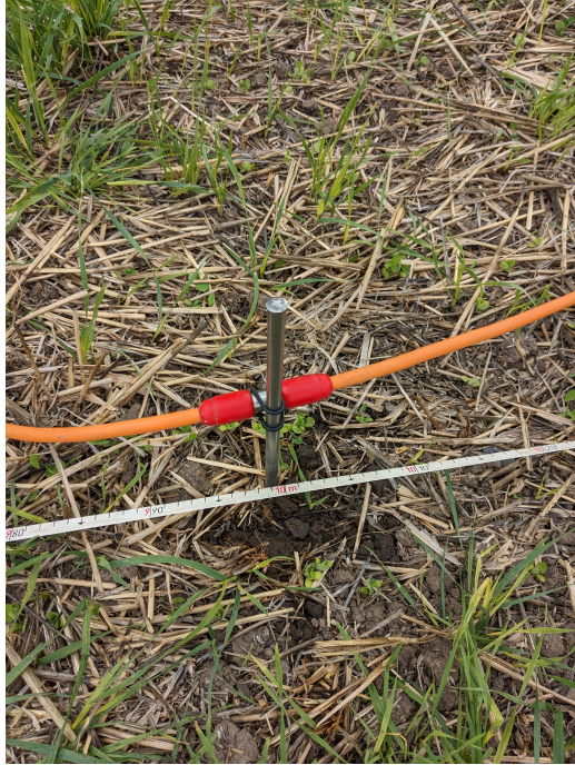
Figure 38: Electrode connected to the wiring
