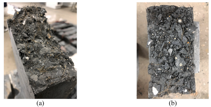
Fig. 8. Fracture surfaces: (a) monotonic loading; (b) cyclic loading.
