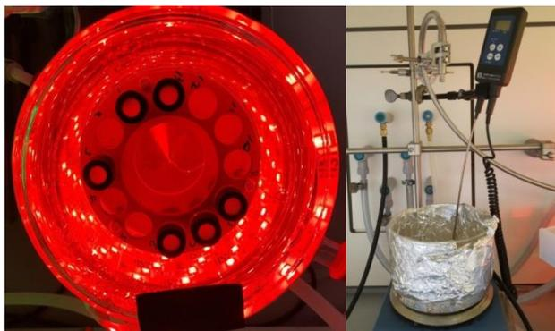
Figure 13. In-house light set up consisting in a jacketed beaker with LEDs winded around (left) and white light set-up consisting on a water bath light beam coming from the top via an optic fibre (right).
