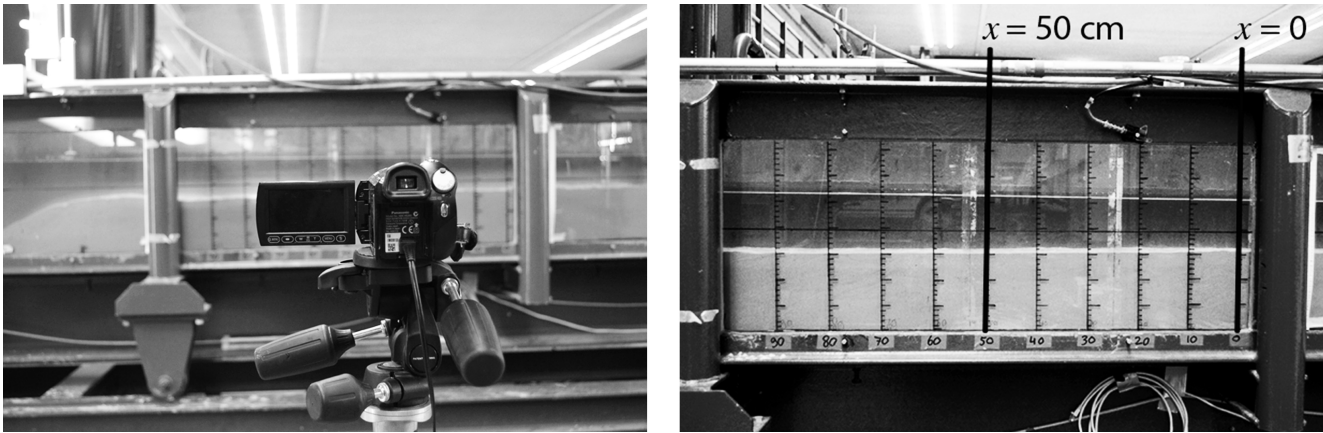
Figure 5. (a) Setup of the camera and (b) Grid on the glass wall in the area of interest.
