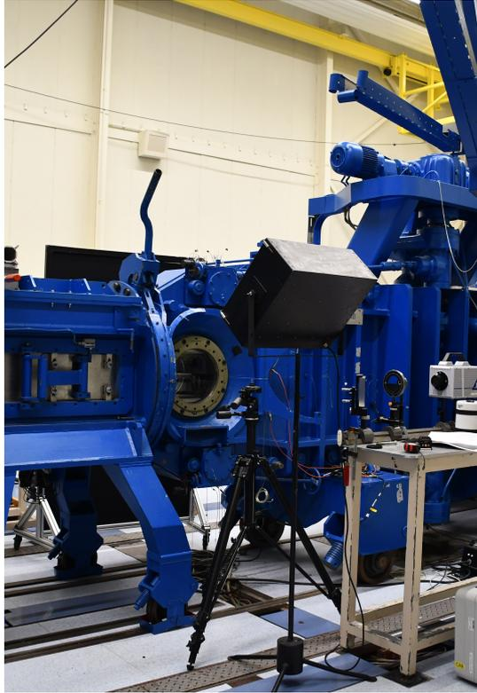
**Figure 3.14:** TST-27 wind tunnel with the tripod and external light system used to record the oil flow runs.
