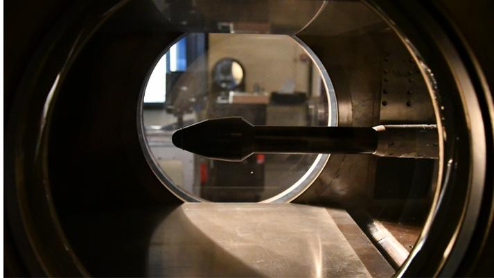
**Figure 3.2:** TST-27 test section with Coe and Nute's Model 11 base geometry configuration, also referred as benchmark configuration along the report. On the background, one of the mirrors used for the z-configuration Schlieren set-up is seen.
