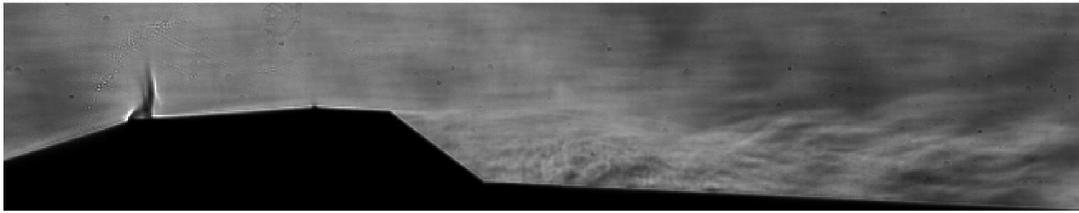
**Figure 4.9:** Instantaneous schlieren image (run 19 at Table B.2) for  $Ma = 0.7$  and  $AoA = 4^\circ$ .
