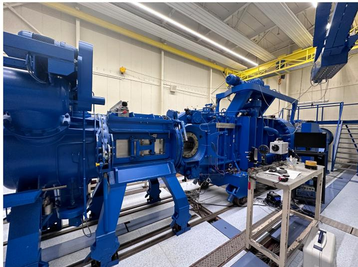
**Figure 3.1:** TST-27 wind tunnel (air flow from right to left) with the Schlieren set-up at z-configuration mounted (table on the right, the last mirrors and lenses together with the camera can be seen from setup described in Figure 3.15).
