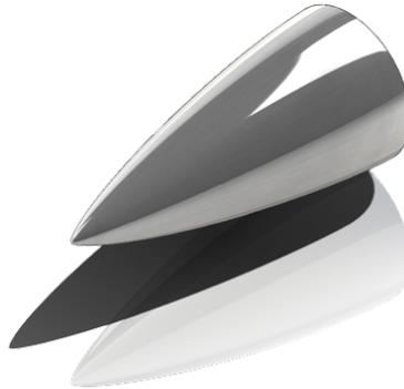
**Figure 2.12:** Sears-Haack minimum drag for given length and diameter series type nose shape (also known as Von Kármán). Source: Wikipedia
