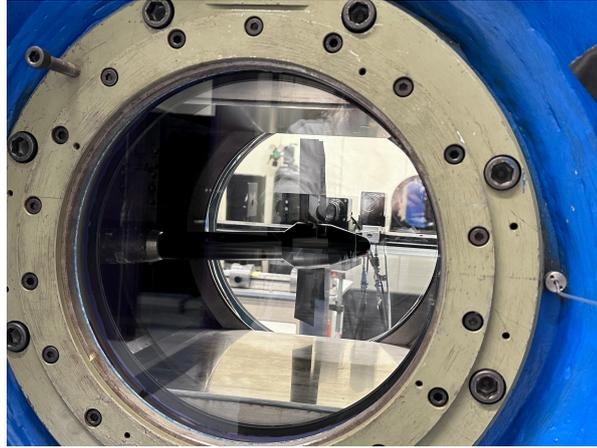
**Figure 3.19:** PIV set-up featuring the benchmark Coe and Nute model positioned at 4 degrees. In the background, two cameras are positioned at different heights to ensure full coverage of the field of view.
