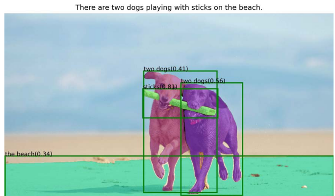
Fig. 15: Semantic segmentation using Grounded SAM [46]. Green bounding boxes are predicted by Grounding-DINO [32] based on the text labels retrieved from the given text prompt, while Segment Anything [29] the corresponding colored segmentation masks.
