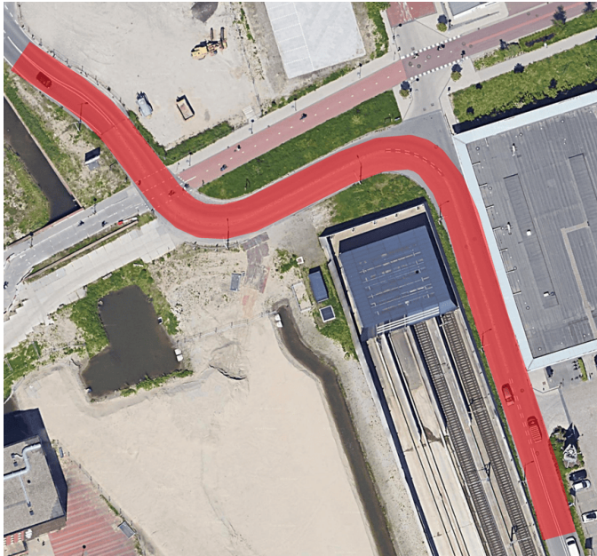
Fig. 24: The final refined road segmentation mask.
