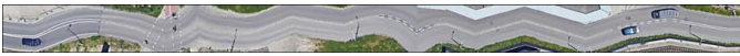
Fig. 17: Example of a normalised road obtained through the piecewise affine warping process.
