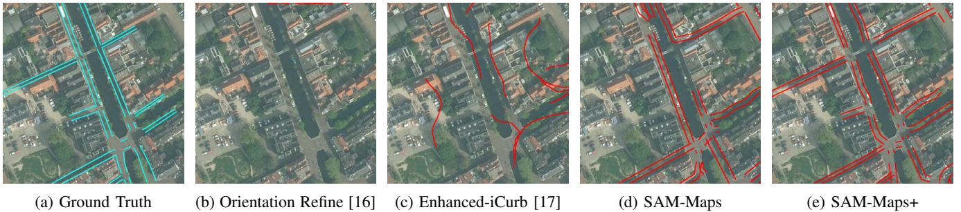
Fig. 26: Qualitative boundary detection results, evaluated on the VoD-P [1] dataset.
