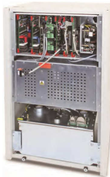
Fig. 1-3 Photo of a HV pulse converter for the X-ray machine [1-15]
