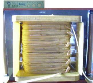
(b) Non-planar barrel HV transformer [2-2]
