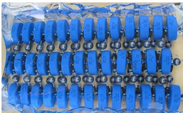
(a) Interconnection by direct soldering
