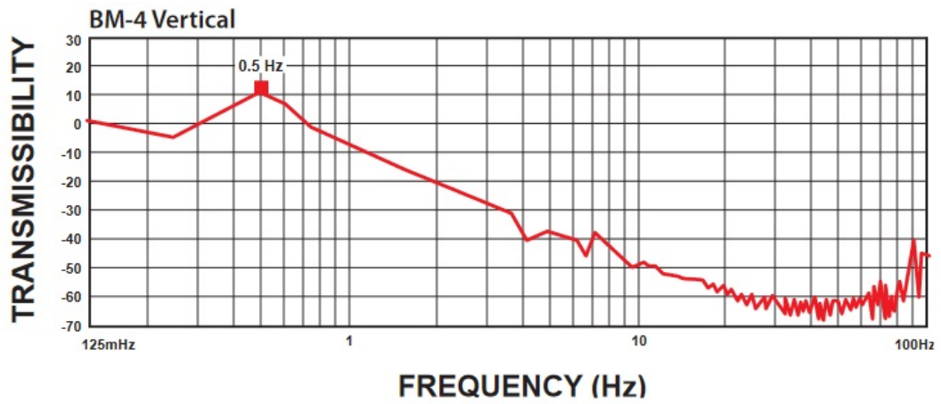
(a) Figure showing the transmissibility of the MinusK 200BM-4 , with the datasheet in C
