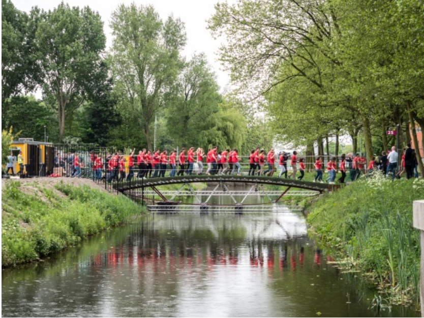
Figure 4. Test loading the Glass Truss Bridge
