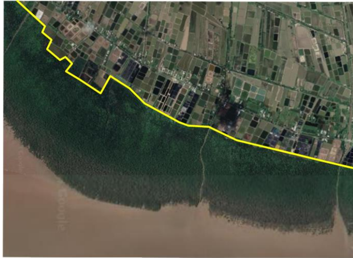
Figure 2.6: Satellite image of mangrove forest and fish farms separated by a dike (in yellow). Image from Google Earth.
